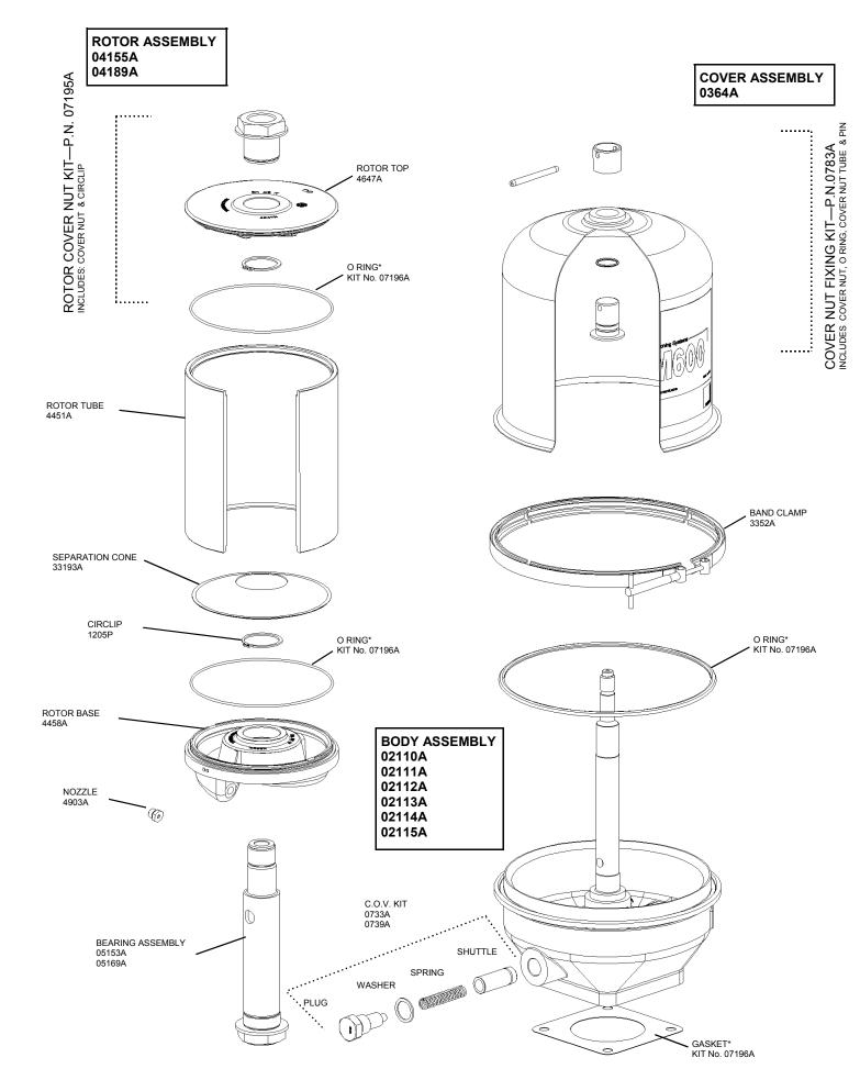
\*SEALS KIT P.N. 07196A COMPRISES OF: C.O.V. WASHER, FILTER BODY O RING, CVR NUT O RING, 2 x RTR BODY O RINGS & BASE GASKET
